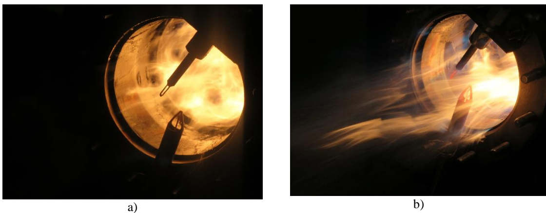
Fig. 9 The fire tube exit: a) 50% camelina oil / 50% kerosene, b) camelina oil
