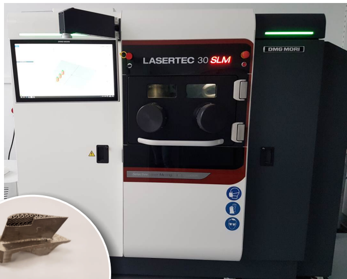
LASERTEC 30SLM Selective laser melting machine with metallic powder.
