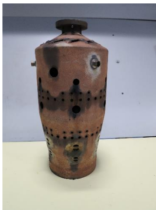
Fig. 1 The fire tube
