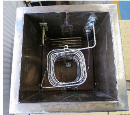
Fig. 5 The oil bath interior
